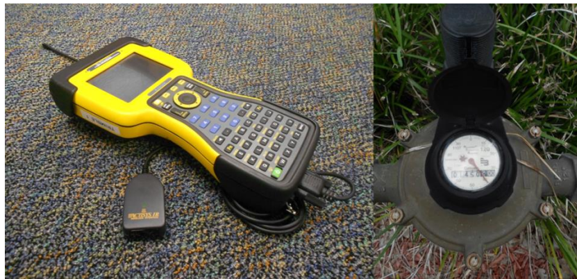
Figure 5.1: Transmitter used for water use data collection (left) and smart water meter (right).
